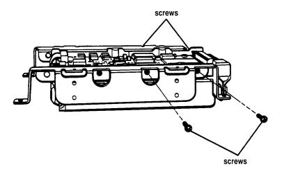
Keep the four screws so you can use them to secure the mounting plate to the hard disk drive. Then set the drive aside with the component side facing up.
